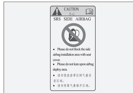
The identification is located on the central pillar. It serves to remind you that the vehicle is equipped with side airbags and to pay attention to the relevant issues.
